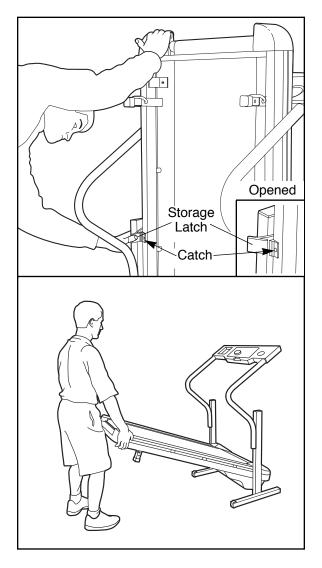
2. Hold the treadmill firmly with both hands, and lower the treadmill to the floor. Do not drop the treadmill frame to the floor. To decrease the possibility of injury, bend your legs and keep your back straight.
